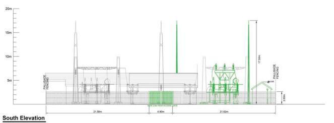
Figure 5.5 - Elevation of the additional plant and apparatus in the existing Woodhouse Substation
